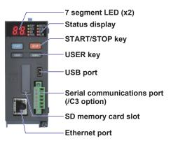
7 segment LED: Displays the operation mode, system No., self-check operation, key lock, operation error, process running, and module installation information.
